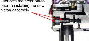
Step 8: Install piston with spring. Attach piston cover plate and then connect pilot line.
