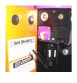
Step 3: Remove the four socket head cap screws holding the piston cover in place.
