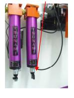
Step 2: Disconnect pilot line from piston cover plate.
