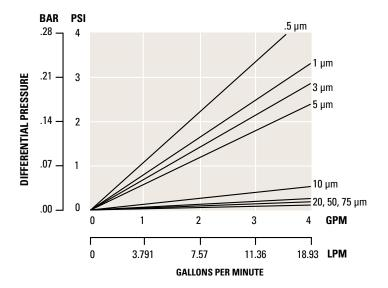
This chart represents typical water flow per 10" cartridge length. The test fluid is water at ambient temperature. Extrapolation for multiple elements tends to be linear, but as flows increase the  $\Delta P$  of the housing becomes more apparent
