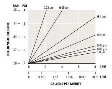
This chart represents typical water flow per 10" cartridge length. The test fluid is water at ambient temperature. Extrapolation for multiple elements tends to be linear, but as flows increase the  $\Delta P$  of the housing becomes more apparent.
