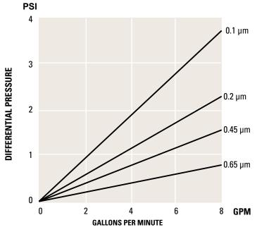
This chart represents the typical water flow per 10" cartridge length. Cartridges are tested in water at ambient temperature. Data may be extrapolated for multiple lengths, but as flow rate increases,  $\Delta P$  of the housing becomes more apparent.
