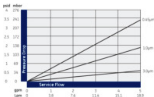
Figure 3: Flotrex medium capsule flow performance in clean water 1
